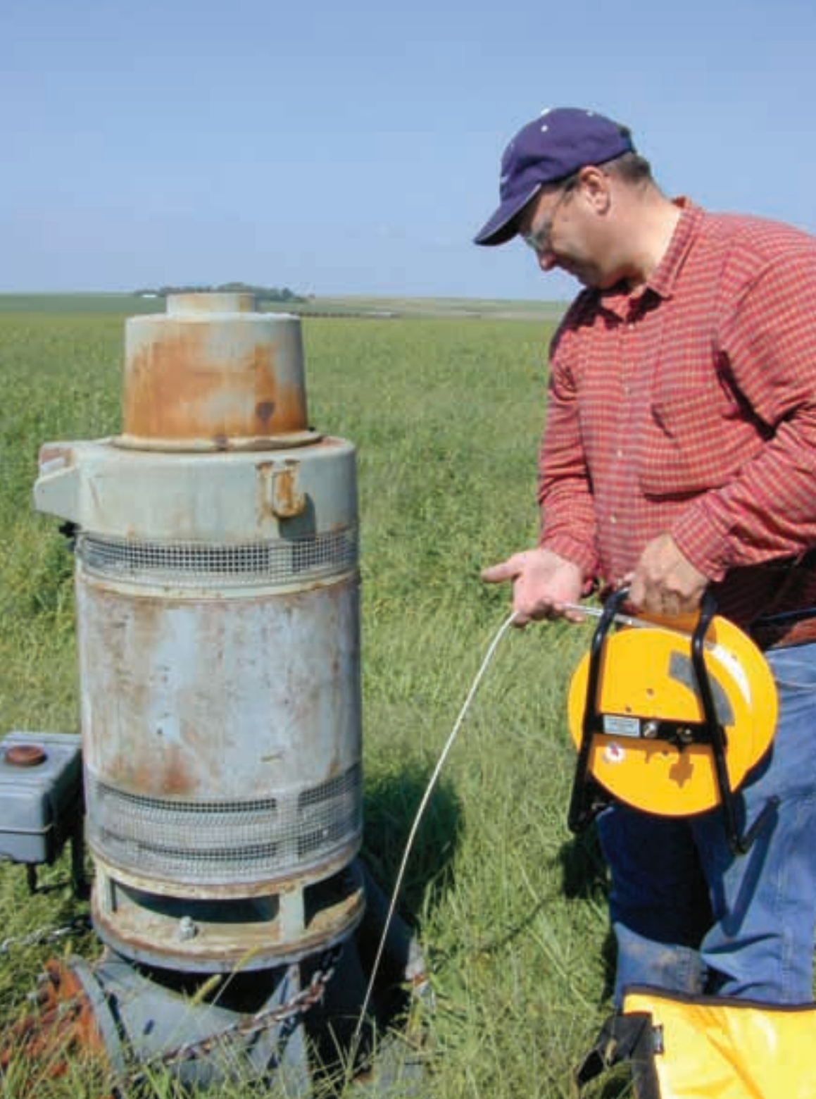
A technician takes a pumping level measurement for a pump-efficiency test on an irrigation well.
