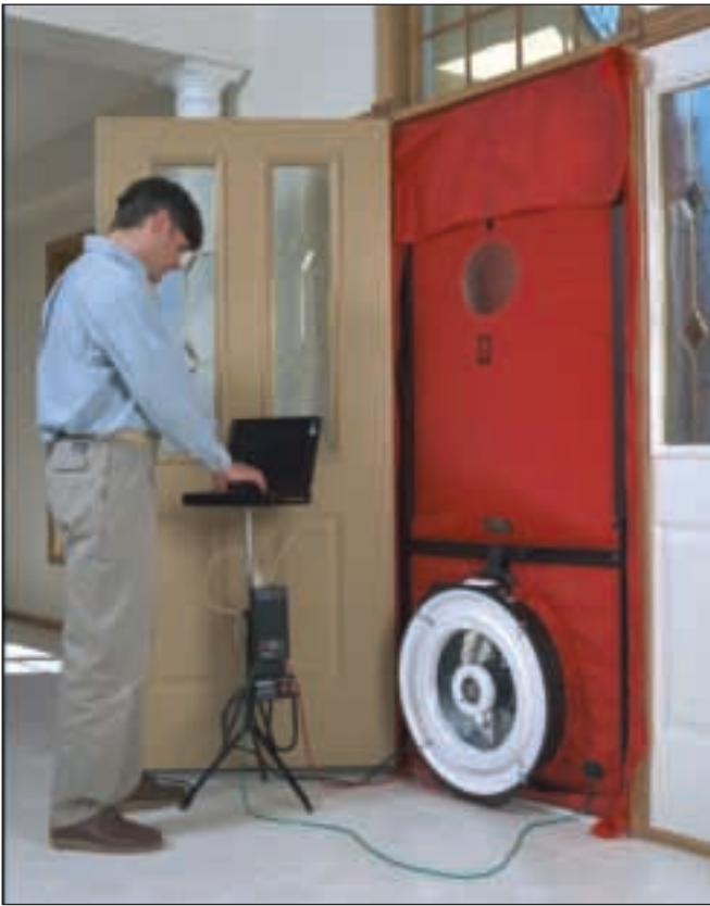
A blower door test determines natural air-infiltration rates.
